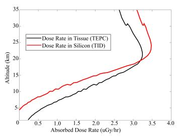
Fig. 11. Comparison of the post-processed absorbed dose rats measured by the TID sensor and the TEPC reference dosimeter
