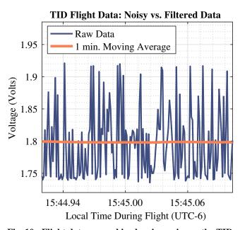
Fig. 10. Flight data zoomed in showing noise on the TID low channel and initial post-processing using a 1 minute average
