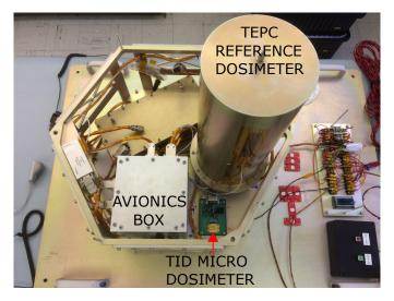
Fig. 3. Overview photo of the RaD-X payload
