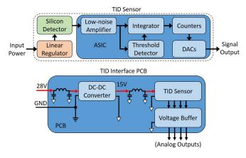
Fig. 4. TID sensor and interface PCB block diagram
