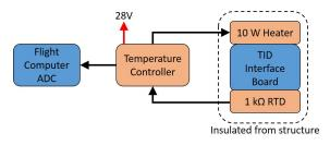
Fig. 14. Active temperature control system block diagram
