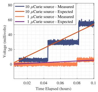
Fig. 8. Lab measurements versus expected results with Cs-137 source, observed noise  $\sim$ 7 mV peak-to-peak
